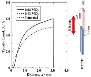
Figure 2: Schematic drawing of shearing test and tensile shear stress ( $\tau$ ) strain ( $\varepsilon$ ) curves at P<sub>s</sub> of PTFE and PE laminated sheet with and without HLEBI at 0.13 and 0.04 MGy at mean P<sub>s</sub> of 0.50.
