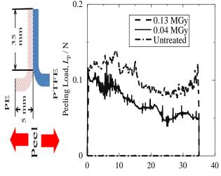
Peeling Distance,  $d_p / mm$  *Figure 1:* Schematic drawing of T-peeling test and adhesive force of peeling resistivity ( $F_p$ ) distance ( $d_p$ ) curves of PTFE and PE laminated sheet with and without HLEBI at 0.13and 0.04 MGy at mean  $P_p$  of 0.50.
